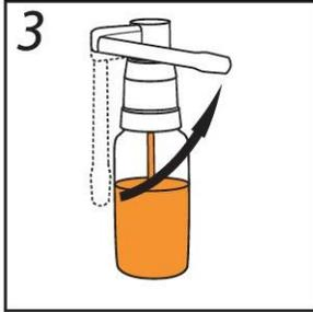
3. Turn the spray nozzle counter-clockwise at a 90-degree angle.
